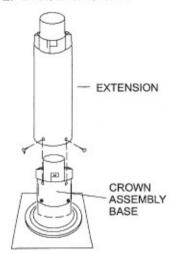
Place the roof jack extension on top of the crown assembly base, pushing down firmly to assure a snug fit. IMPORTANT: Make sure that the pipes are connected.
