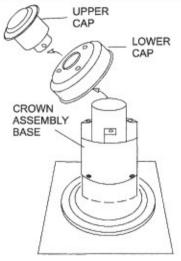
Remove the 2 screws that secure the upper cap to the crown assembly base and remove the upper cap. Next, remove the 3 screws that secure the lower cap to the crown assembly base. Set both caps aside for later use.
