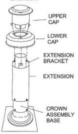
Using the 3 screws removed in step 3, attach the lower cap to the extension bracket. Install the upper cap over the center pipe of the extension. Using the 2 holes located at the base of the upper cap as guides, drill 2 holes 1/8" diameter into the center pipe. Finally, attach the upper cap to the center pipe using the 2 screws removed in step 3 to the center pipe.
